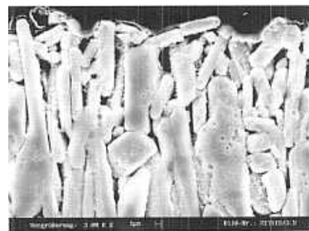
Abb. 11f: A_s = 42,7 \mu\text{m/min} , 0,32 \% Si, 460^\circ\text{C}
